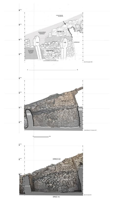
Figure 7. L09-80 elevation of wall L09-80-65/15 and 144 (hand drawing 2002 by D. Kurapkat, 3D-model 2017 by M. Kinzel, D. Sönmez, 3D-model 2018, by M. Kinzel, edited by M. Kinzel 2020).
